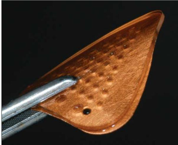
**Figure 3.** Poly lactide plate after heating in water.
