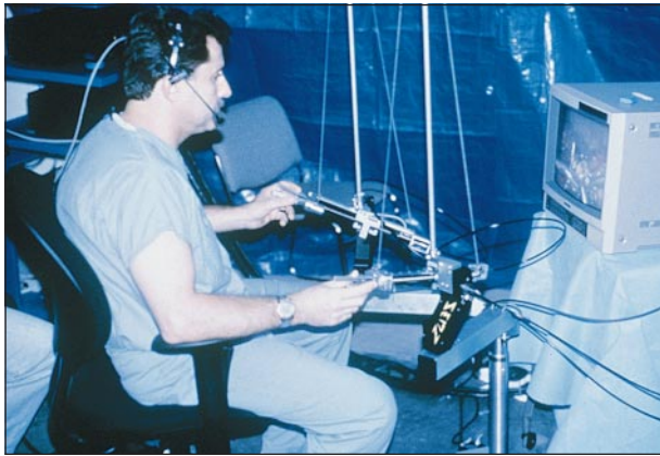
Figure 3. The Zeus telesurgery system for enhanced microsurgery. (Courtesy of Yulun Wang, MD, Computer Motion Inc, Goleta, Calif.)
