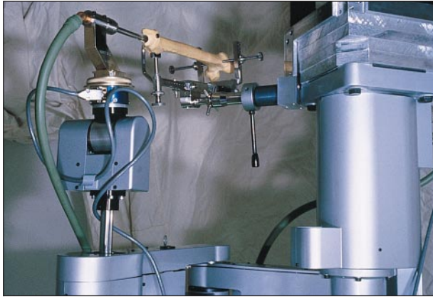
Figure 2. The precision surgical robot, Robodoc (Integrated Surgical Systems, Davis, Calif), for high-precision hip replacement surgery. (Courtesy of William Barger, MD, University of California, Davis, Sacramento.)
