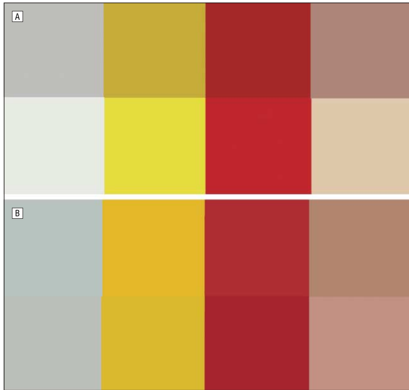
Figure 2. Comparison of some colors between the 2 most divergent uncalibrated images of the MacBeth ColorChecker Chart (GretagMacBeth, Regensdorf, Switzerland), before (A) and after (B) calibration.
